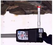
Quick Measure can perform several special functions: symmetry measuring, cross measuring, distance and width measuring etc. which help the body shop to accomplish a wide variety of jobs in minimum time.
